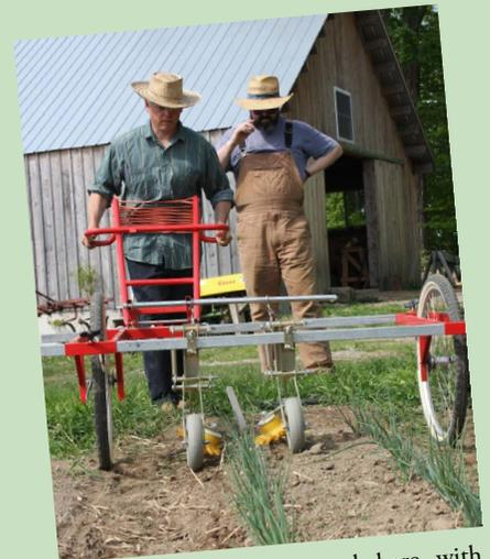
The 'Weedmaster,' pictured here with finger weeder attachments, is a versatile person-powered cultivator that can also be equipped with disk hillers, sweeps, and flaming equipment.
