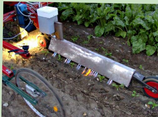
This robotic flame-weeder is mounted with a camera that distinguishes between weeds and crop plants, allowing it to automatically toast inter-row weeds.
