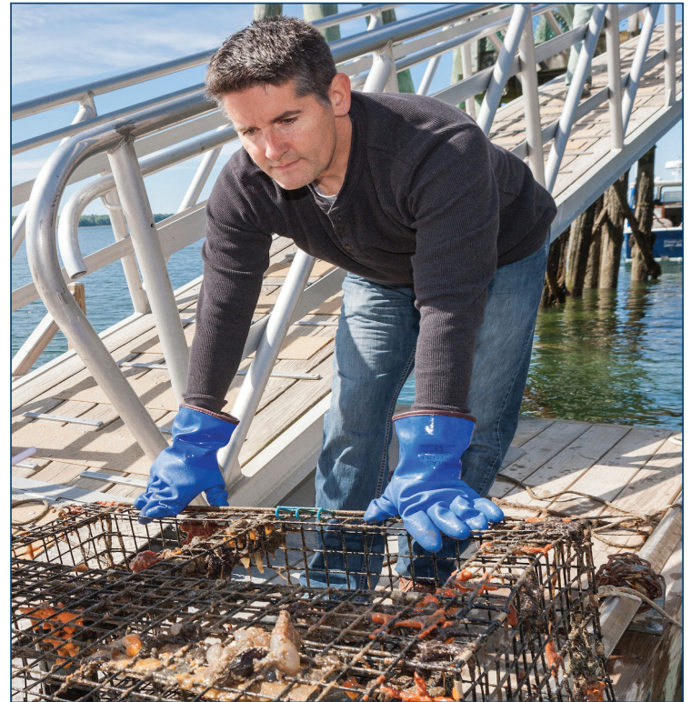
Marine Life Mike Doan, Friends of Casco Bay Research Associate, hauls up the Cage of Science—electronic equipment housed in a converted lobster trap that records hour-by-hour data on the bay’s temperature, carbon dioxide, oxygen, pH, salinity and chlorophyll. (KEVIN MORRIS PHOTO)
