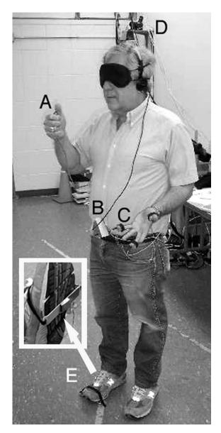
Figure 1. Apparatus for the navigation task: (A) push button, (B) body orientation sensor, (C) vibrator on finger, (D) head orientation sensor, (E) footstep sensor (also shown in inset).
