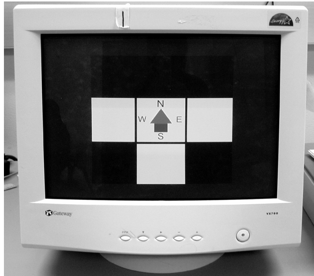
Fig. 3. Sample 3-way intersection as seen on a visual display. Information seen from each view is matched to what would be heard in the corresponding message from the VVD.
