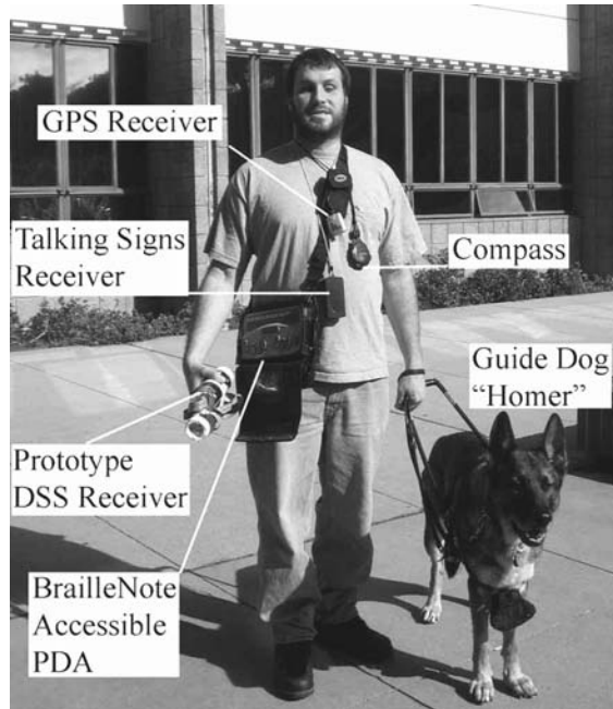
FIGURE 25.1 A blind pedestrian is using a guide dog and five technologies for navigation. This figure illustrates the need for an integrated navigational system. The guide dog aids with mobility and obstacle avoidance. The compass provides the user with heading information when stationary. The GPS receiver integrates with a GIS database (digital map) to provide position and heading information during outdoor navigation. The talking signs receiver gives orientation cues by identifying the direction and location of important landmarks in the environment. The digital sign system (DSS) receiver picks up barcodes from signs and sends them to a database to facilitate indoor navigation. The BrailleNote accessible computer represents the “brain” of the system, allowing Braille input and speech and Braille output. In theory this device could serve as the hub to which all other technologies interface.
