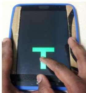
Figure 3. Subject tracing stimuli displayed on the touch-based device with the vibro-audio mode.
