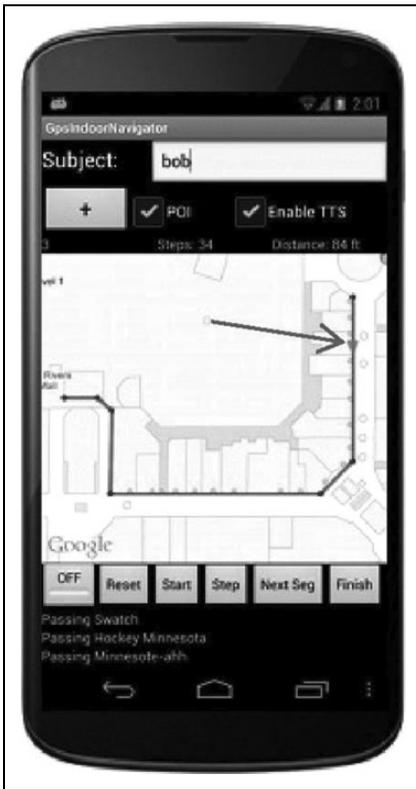
**Figure 3.** Navigator application running on a Nexus 4 smartphone, showing users current position estimate. *Source:* Reprinted with permission from Riehle, Anderson, Lichter, Whalen, and Giudice (2013; ©IEEE 2013).
