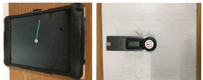
Figure 8. Randomly generated oriented lines rendered on the experimental device and (right) the digital pointing device used for reproducing line orientation.
