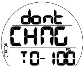
If in decompression and a better gas is available based on your PO<sub>2</sub> alarm settings, your Veo 4.0 will prompt you to switch gases. You may confirm the gas switch by pressing SEL while the gas switch prompt screen is displayed. If not confirmed the, the Veo 4.0 will restore the Dive Main screen without switching gases. You may still switch gases manually after the prompt clears if you choose to do so.
