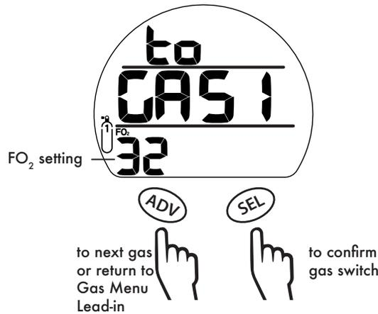
If the current PO<sub>2</sub> value is greater than 1.6, then a warning not to switch will display. The Veo 4.0 will maintain the current gas without switching. The diver may override the Veo 4.0 and force the gas switch by pressing the SELECT button during the "dont CHNG TO-" message.
