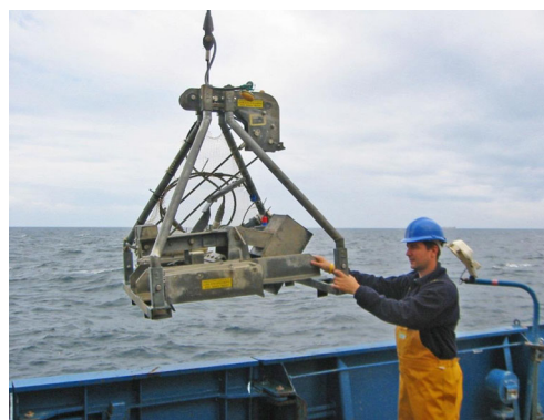
Fig. 2 A Hamon type grab sampler operated on board of an oceanographic ship (Source: Modified from Wessex Archeology)
