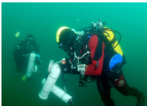
Fig. 1 CRALF water sampling bottle was specifically designed to allow scuba divers collecting water samples in situ in glacial lakes (Source: Pardo and Rodríguez 2007)
