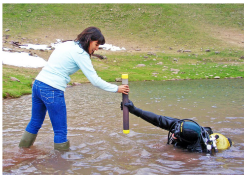
Fig. 9 Push-cores handling must be careful during the sampling and transport processes. At no time during the underwater carriage or its surface collection, a core has to lose its original orientation. Turning it over or even a mild shake would cause disturbance or destruction of the sediment lamination rendering a useless sample for certain paleolimnological and sedimentary analyses (photograph Tomás Arribeo)
