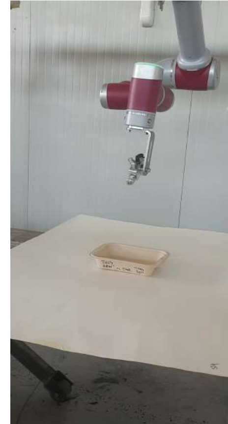
Spray gun moving around the 3D MF tray, according to the programmed trajectory.
