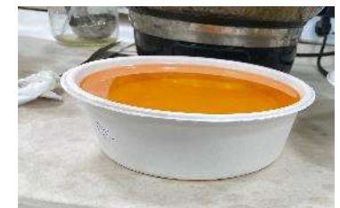
Hot Oil Test: 1L, 100°C, Pass
