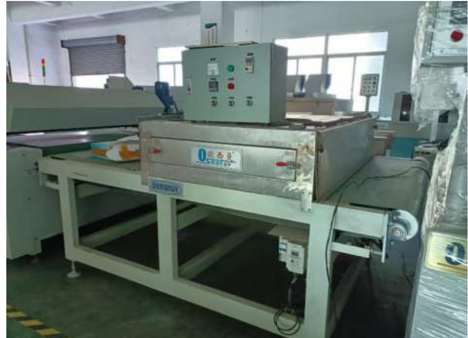
IR dryer, with conveyer belt
