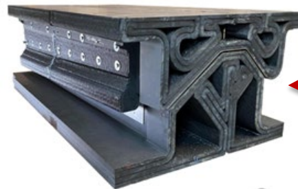
AM Mold with Metal Cladding 60" long x 32" wide x 21" tall
