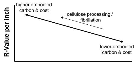
**Fiber Diameter or Insulation Pore Size**
