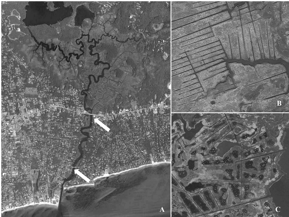
Figure 2.1. Examples of direct tidal marsh modifications by humans. A) tidally restricted marsh (white arrows show individual restrictions), B) ditched marsh, and C) marsh treated with Open Marsh Water Management (OMWM).
