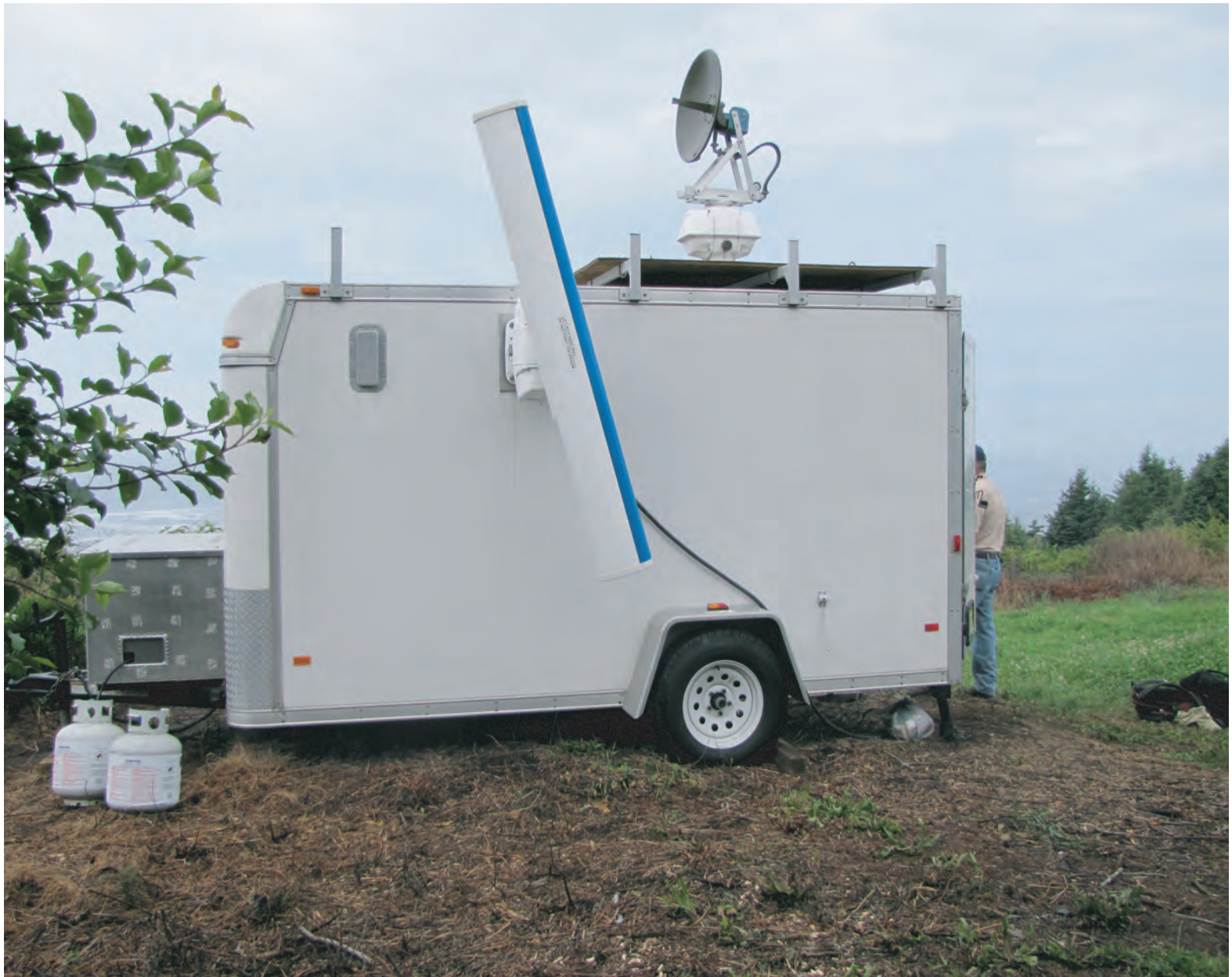
Figure 1. Dual radar system with vertically-oriented (open-array) and horizontally-oriented (parabolic dish) antennas that operate simultaneously. This system allows for data collection on passage (horizontal and vertical), altitude (vertical) and flight direction (horizontal).
