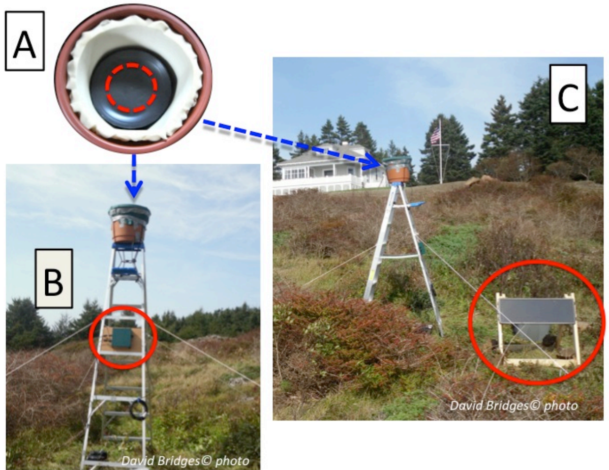
Figure 5. The microphone assembly (A, microphone element noted with red hatched circle) was covered by thin cotton cloth (green, as shown in B), directed skyward, and, along with the Wildlife Acoustics SM2 ® recorder (shown within the solid red circle in B), was anchored firmly to the stand. A 12-V battery (at base of ladder in B) charged by a solar panel (in solid red circle in C) supplied power.
