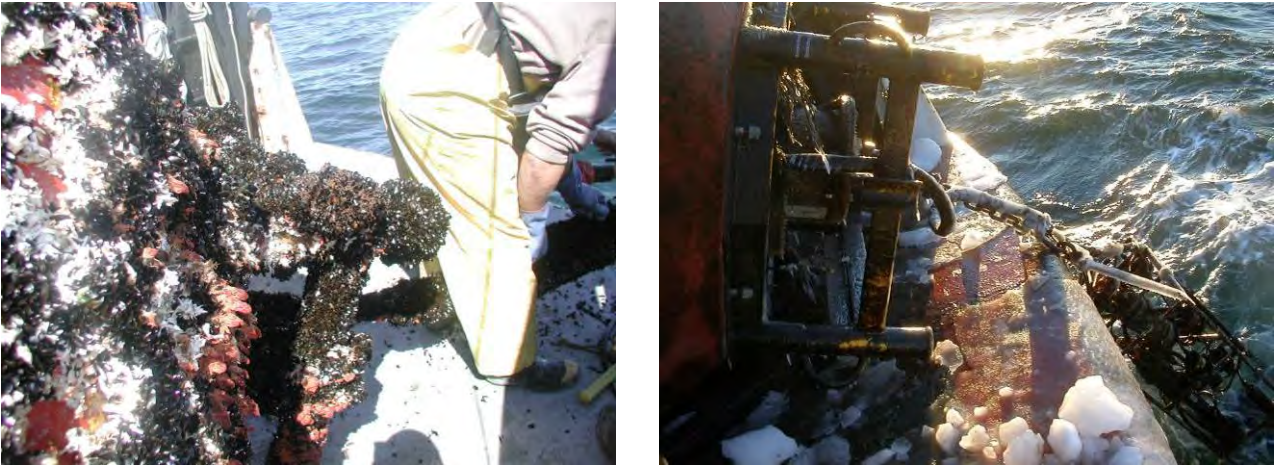
Figure 1-2 Representative biofouling on Gulf of Maine Oceanographic Buoys. Buoy E01 summer fouling shown on left and Buoy E01 winter fouling shown on right
