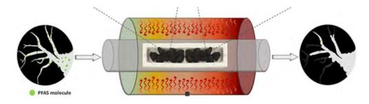
Activated carbon thermal regeneration image from Baghirzade et al. (2021)
