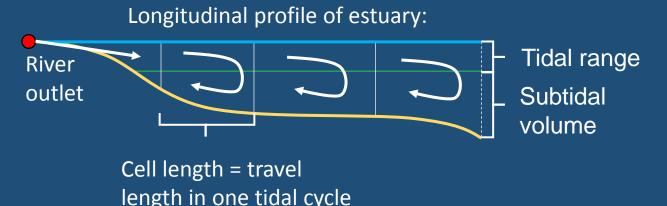
Estimate the capacity of an estuary to flush contaminated water by tidal power (Ketchum, 1951)
