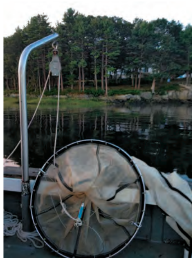
FIGURE 4 Plankton tow net used to collect larval fish at multiple locations within the Saco estuary.
