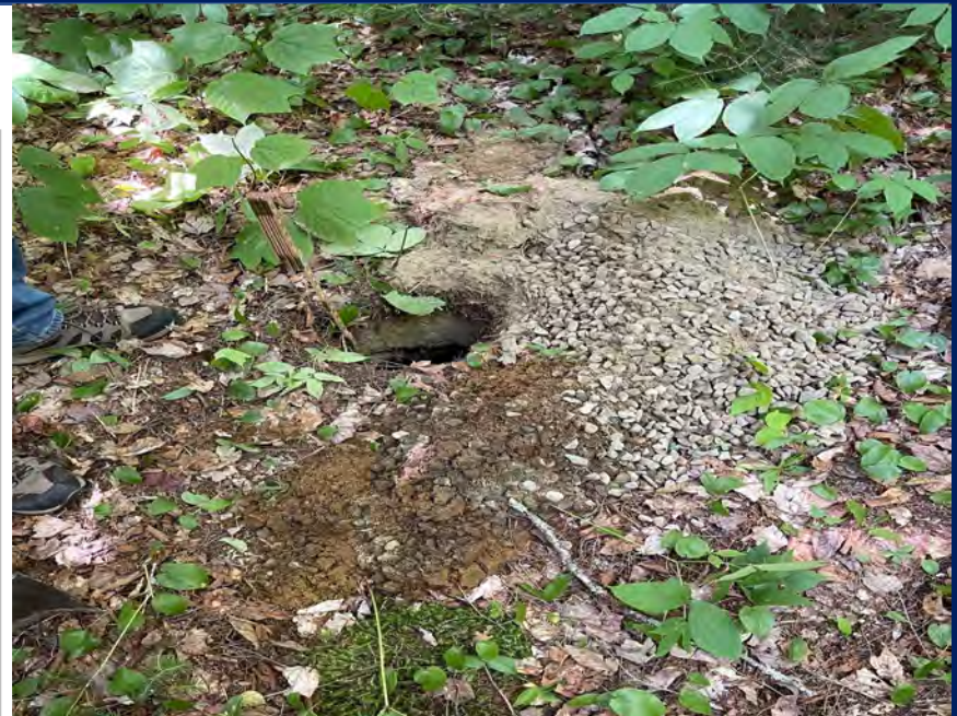
Clean stone- no evidence of Biomat
