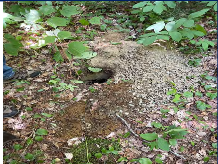
Clean stone- no evidence of Biomat
