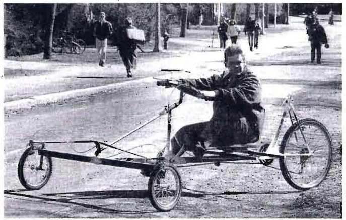
The University of Maine's Mechanical Engineering Technology students are designing and building amphibious vehicles as their annual senior projects. Jason Spencer of Passadumkeag makes a test run with his vehicle which will be entered in the 1993-94 Human Powered Amphibious Vehicle Competition on Saturday, April 30, in the Stillwater River and on the UMaine campus. Styrofoam will be added to the vehicle to provide buoyancy for the river portion of the competition. Photo by Monty Rand
