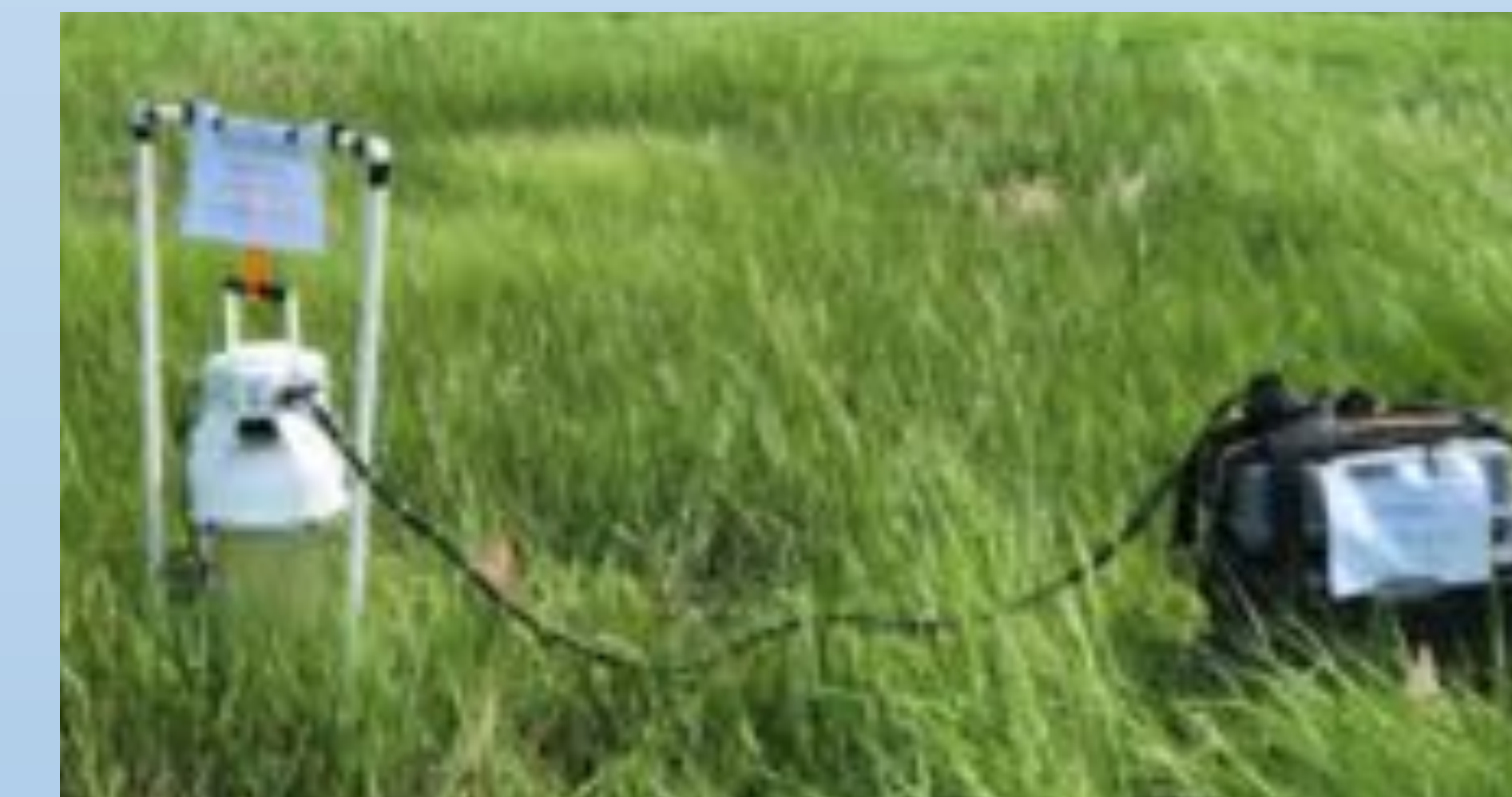
Figure 3. LICOR-7810 greenhouse gas flux analyzer (on right) with SMART chamber and collar (on left), setup for a 24 hour data collection
