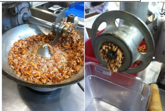
Figure 4. Cutting and grinding cooked lobster shell for subsequent astaxanthin extractions.
