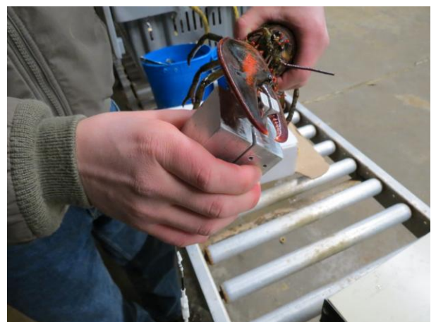
Measuring lobster grip strength using a prototype load cell.
