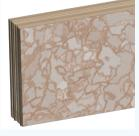
Laminated & Oriented Strand Lumber (LSL; OSL) Parallel layers of long (LSL) or short (OSL) length-to thickness stranded wood flakes joined using glue to form beams and columns.
