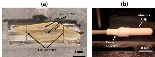
**Fig. 24. (a) Top-view of a LGS SAWR sensor device attached and electronically connected to a high temperature Inconel cable. (b) The same device shown in (a) packaged/protected with an alumina cap using a high temperature ceramic adhesive. Reproduced from [3].**
