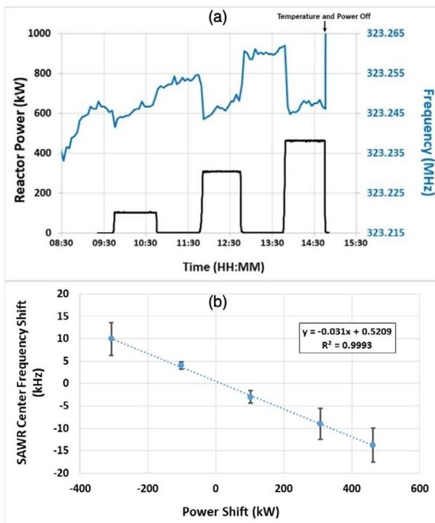
**Fig. 26. (a) Representative LGS SAWR sensor with Pt-Al<sub>2</sub>O<sub>3</sub> electrodes showing frequency response at 800°C versus different reactor power levels. (b) Average frequency shift versus reactor power shift. Reproduced from reference 3.**
