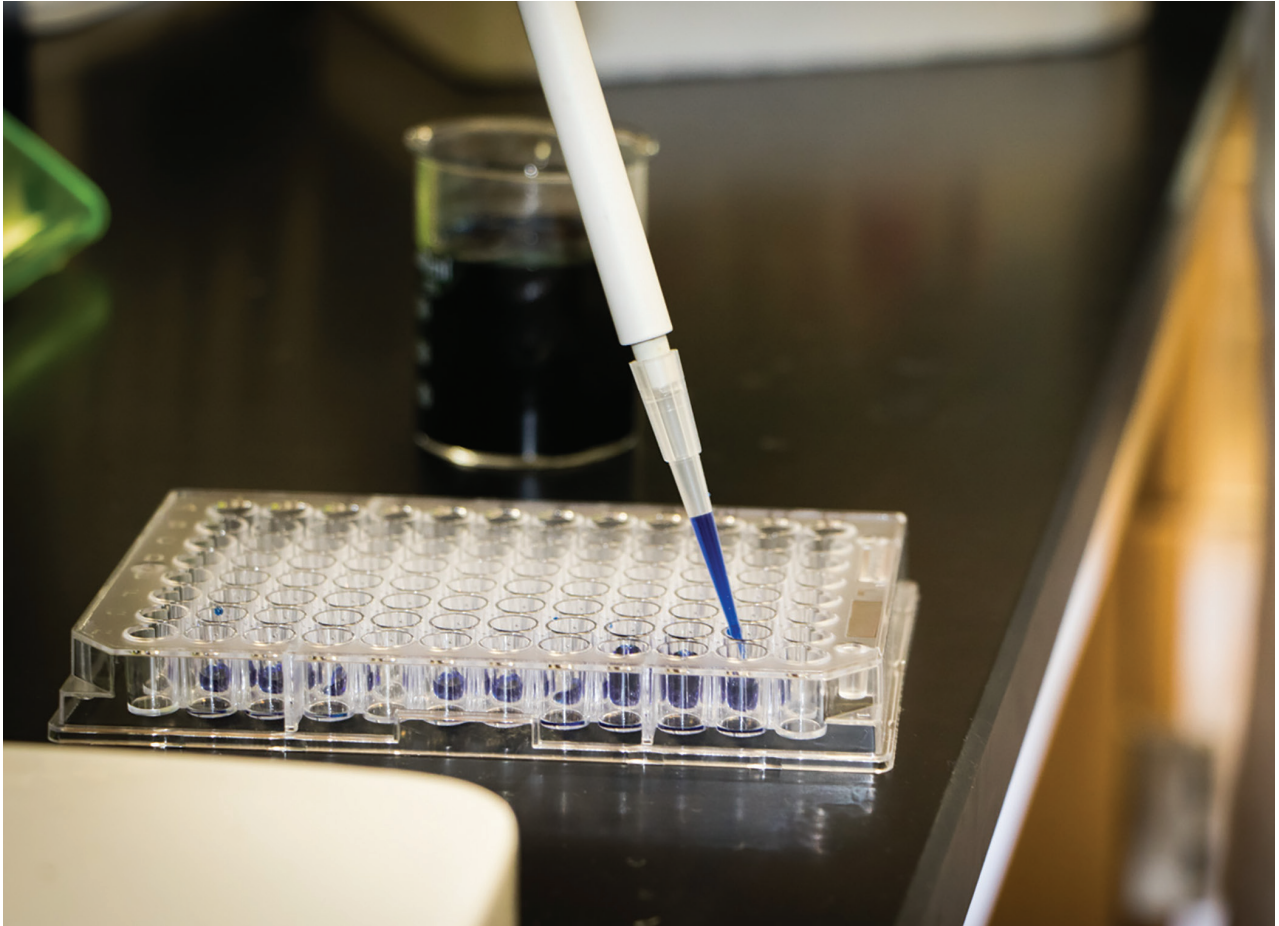
Analysis of the antioxidant capacity of post-processed seaweed using a colorimetric assay.
