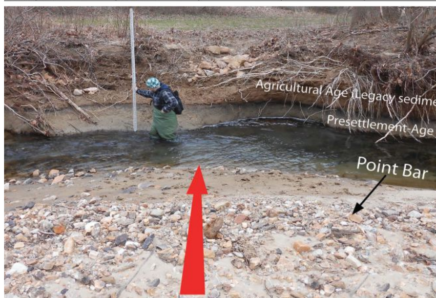
This photo is of the lead author in the Donovan study surveying a stream cross-section. Note the "legacy sediment" (erosion from agriculture) on top of the pre-settlement deposits. The stick figure in the diagram on top indicates where the photograph was taken. Photo courtesy M. Donovan, A. Miller, M. Baker and A. Gellis
