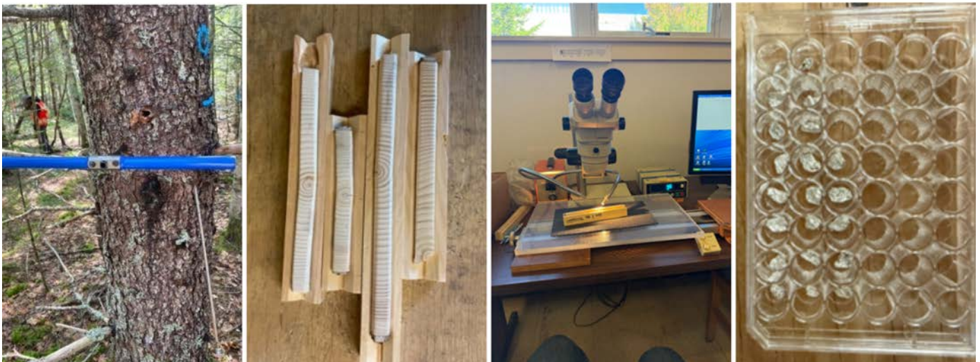
Figure 1. Increment borer sampling at the Penobscot Experimental Forest Installation (far left), the 0.5-inch diameter increment cores mounted for cross-dating at the dendrochronology laboratory middle right, where individual tree rings are ground and processed in the Forest Management Lab at the University of Maine for later analysis at Columbia University (photos courtesy of Lila Beck)
