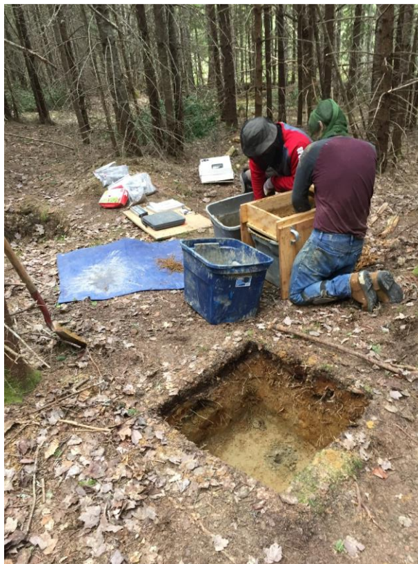
Quantitative soil pit excavation on a moderately well drained (MWD) site. Sieving and weighing of soil samples was conducted by field crew members Keegan Ferro and Chris Preece.
