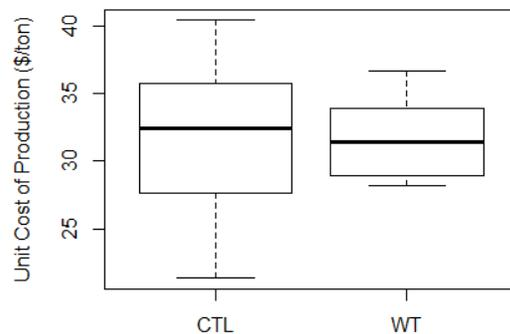
**Figure 2-10.** Variation in unit cost of production (\$/ton) for WT and CTL systems. Bold lines represent median unit costs.
