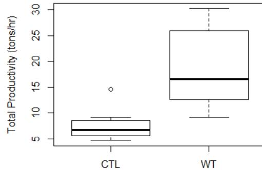
**Figure 2-9.** Variation in machine-level productivity (tons/hr) for feller bunchers (WT) and processors (CTL). Bold lines represent median productivity.
