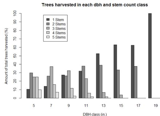
**Figure 2-13.** Percentage of trees harvested in each dbh class for all five stem count classes in feller-buncher head accumulations (n=949).
