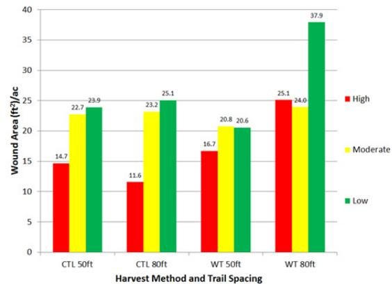
**Figure 2-6.** Wound area (ft<sup>2</sup>/ac) separated by severity class and shown by harvest method and trail spacing.
