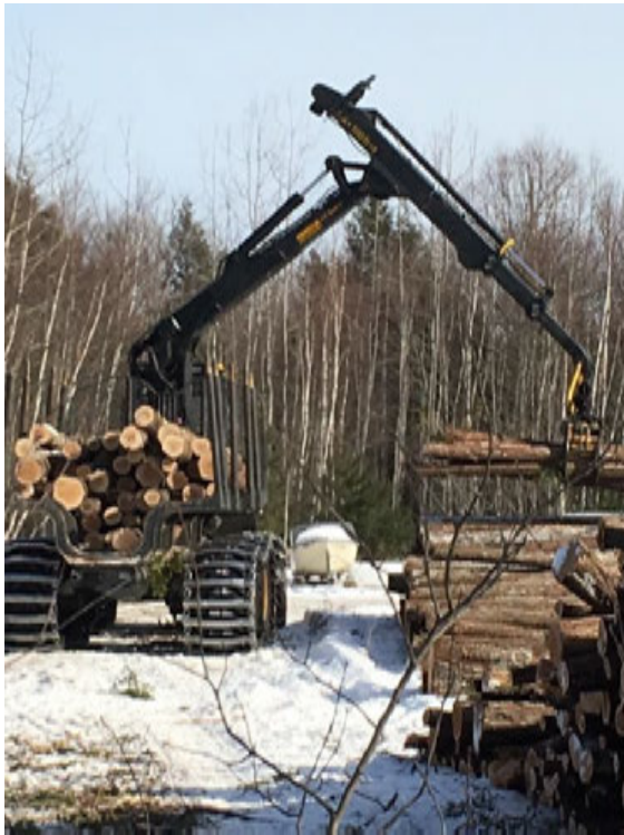
Photo 2. Buffalo Forwarder piling white-cedar logs at the landing on the PEF.
