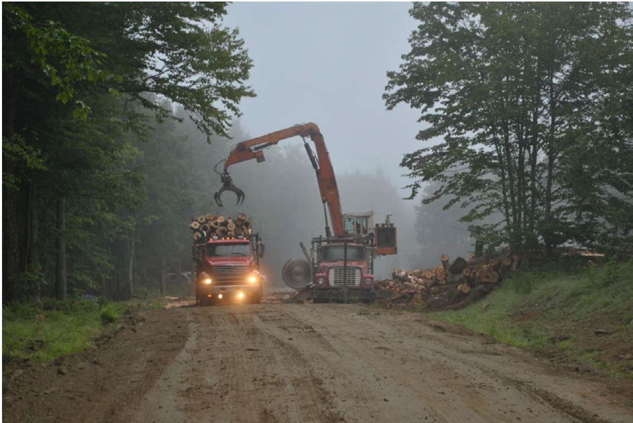
Photo 2. Slasher loading log trucks at the Grand Falls Operation.
