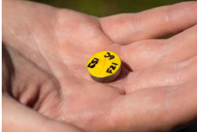
Photo 2. The picture above shows an example of an iButton temperature monitor used to track ambient temperature data in and around the nest site.
