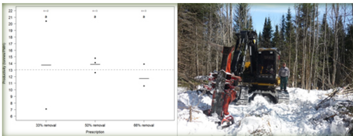
Figure 6 - [left] Feller-buncher productivity across three different prescriptions. Black lines represent the average harvester productivity for each prescription. The gray dashed line represents the overall mean. Letters at the top of each prescription s show statistically different means. [right] CAT 501 feller-buncher with operator Brian Mack in a non-PCT stand (right). Photo credit: Patrick Hiesl.
