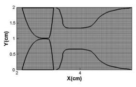
FIGURE 4. Grid used in the vicinity of vocal folds and false vocal folds in the current simulations.
