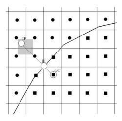
FIGURE 2. Schematic of the immersed boundary representation in the current method. IP, image point, GC, ghost point, BI, boundary intercept point.
