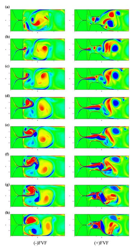
FIGURE 12. Contours of spanwise vorticity for the two cases over one vocal fold vibration cycle. The eight plots correspond to eight equispaced time intervals over the vibration cycle.
