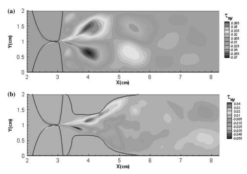
FIGURE 14. Contours of fluctuation shear stress in the glottal jet. (a) (-)FVF case, (b) (+)FVF case.
