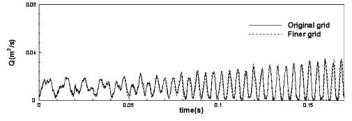
FIGURE 7. Comparison of flow volume flux rate for original grid and finer grid.
