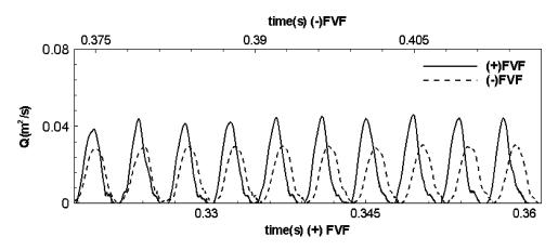
FIGURE 10. Comparison of the time variation of the volume flow rate for the two cases.
