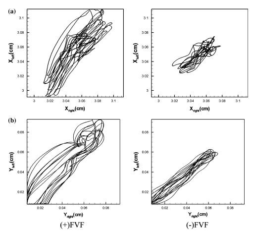
FIGURE 16. Phase plane plots of the displacement of the points on the superior side of the two vocal folds. (a) x displacement (inferior-superior), (b) y displacement (abduction-adduction) from centerline.
