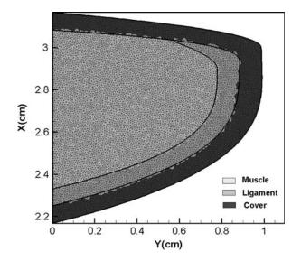
FIGURE 5. Three layer vocal fold inner structure and triangular elements used in the current solver.
