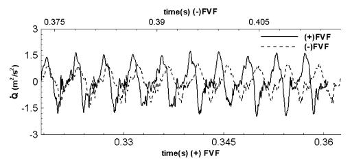
FIGURE 11. Comparison of the time-rate of change of the flow rate, Q, for the two cases. This quantity is related to the monopole source strength of sound.
