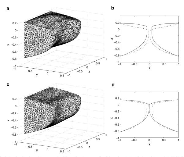
Fig. 9. The eigenfunctions of first two modes (left panel) and corresponding deformations in the mid-plane (right panel). (a, b) Mode-1, 114 Hz and (c, d) mode-2, 125 Hz.
