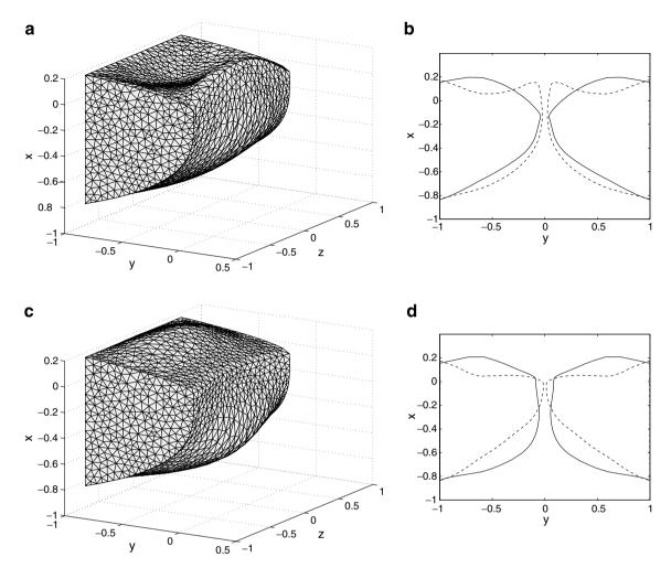
Fig. 10. The eigenfunctions of mode-3 and 4 (left panel) and corresponding deformations in the mid-plane (right panel). (a, b) Mode-3, 133 Hz and (c, d) mode-4, 144 Hz.
