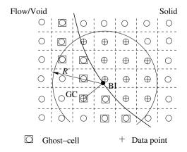
Fig. 5. Treatment of the traction boundary condition.
