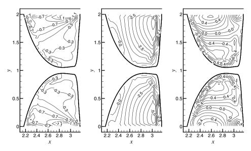
Fig. 23. Stresses in the vocal folds as they are fully open ( $\eta = 10$  p). (a)  $\sigma_{xx}$ ; (b)  $\sigma_{yy}$  and (c)  $\sigma_{xy}$ .
