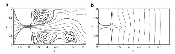
Fig. 22. Averaged flow field between t = 18 cs and t = 25 cs for  $\eta = 10$  p. (a) Streamlines and (b)  $v_1$  velocity profiles at different locations. Every 1 cm represents a velocity of 50 m/s.
