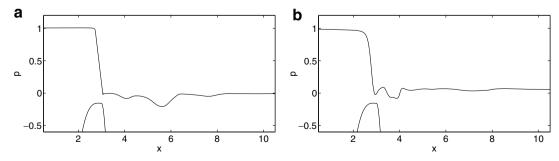
Fig. 19. Gage pressure (kPa) along the centerline of the channel for  $\eta = 10$  p. (a) t = 18.20 cs (closure phase) (b) t = 18.40 cs (open phase). The streamwise position of the vocal fold is also shown.
