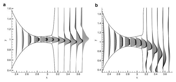
Fig. 20. Instantaneous velocity field around the glottis during the open phase for (a)  $\eta = 10$  p and (b)  $\eta = 6$  p. Only partial grid points are shown.
