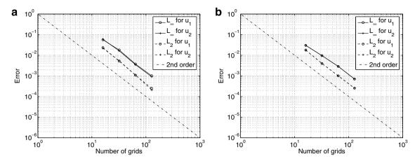
Fig. 7. Error norms of the solution obtained using the immersed-boundary method for the plane-strain annulus case with (a) traction-free inner surface and (b) fixed inner surface. The dash-dot line represents the second-order convergence rate.
