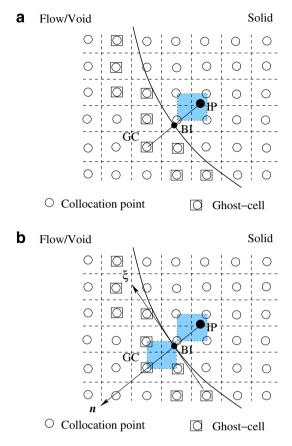
Fig. 4. Schematic of the immersed-boundary method on a Cartesian grid for solving the linear viscoelasticity. The bold curve represents the boundary of the solid. The stencil is shown in (a) for the displacement boundary condition and in (b) for the traction boundary condition.
