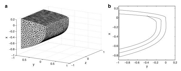
Fig. 8. (a) A 3D view of the vocal fold model. (b) The coronal section which consists of, from outside, the cover, the ligament, and the body. The length unit is centimeter.
