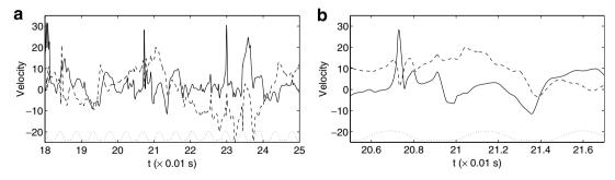
Fig. 21. Histories of  $v_1$  (m/s) (solid lines) and  $v_2$  (dashed lines) at x = 4.5 cm on the centerline. A close-up is shown in (b). The dotted lines represent the phase of the glottal gap.
