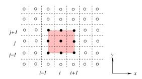
Fig. 2. The stencil that is used in the IB method to discretize the field equation at the collocation point (i,j). The nodal points involved in the stencil are marked with filled circles, while other nodal points are marked with unfilled circles.
