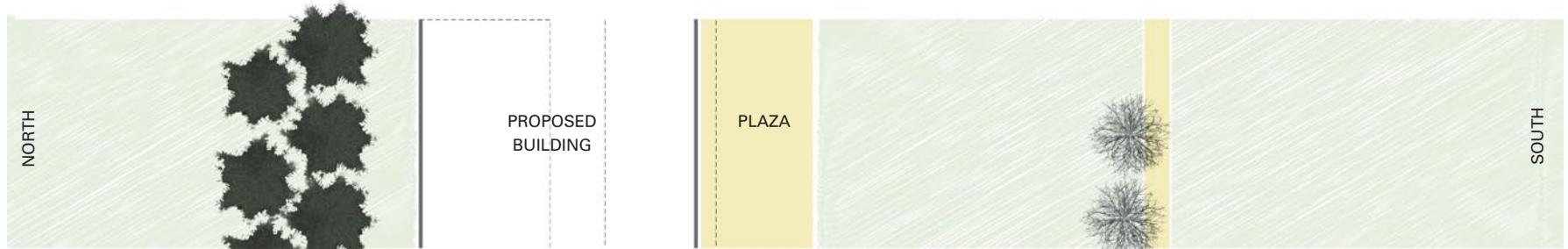
SECTION OF OPTIMAL BUILDING ORIENTATION SHARING WINDBREAK AND SHELTERED SOUTHERN OUTDOOR SPACE
