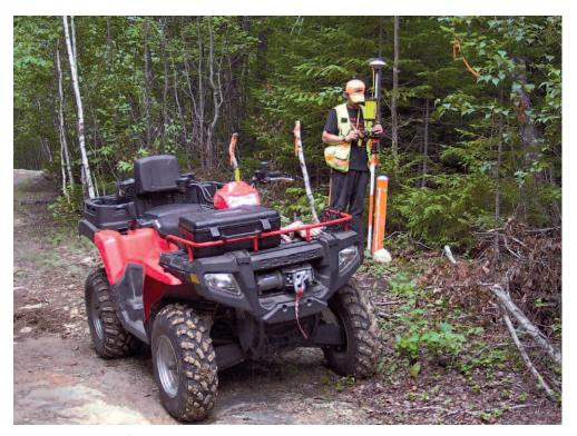
Surveyors work in a variety of unique outdoor locations. This surveyor is using a data collector and survey grade global positioning system receiver to communicate with satellites for extremely accurate land measurements.
