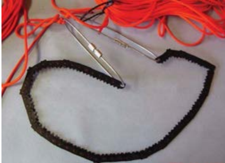
Figure 12. Example of a rope saw provided by US Forest Service (Mason 2010).
