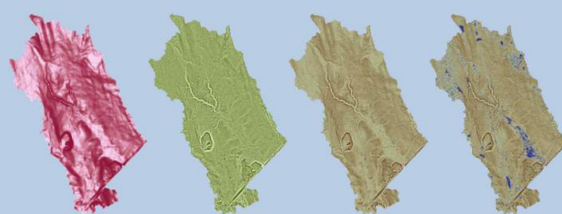
Figure 5. LIDAR derivative layers showing slope (low-high: light-dark purple), TPI (neg-pos: light-dark green), slope-TPI visual overlay (lightest browns are flattest slopes and most negative TPIS); overlay with storage
