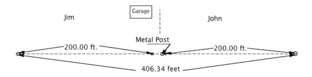
As the diagram shows, the metal post falls within the realm of possibilities given the vague deed description (though not an equal allotment of the excess). While the post may not be where a surveyor would place the common corner, the post does fall within the realm of possible locations fixed by the deed description. As such, the courts would tend to favor the position of the post as the deed corner simply because the parties-in-interest have historically done so.
