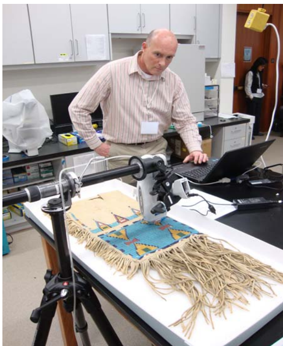
Conducting pXRF analysis of beads in his laboratory.
